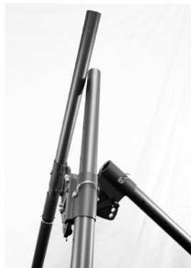
Fig 8 Rear leg with centered leg clamp. Legs are able to by-pass each other due to offset leg clamp orientation
