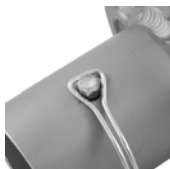
Fig 2 Properly Secured Leg Coupling Pin
