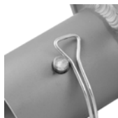
Fig 3 Improperly Secured Leg Coupling Pin
